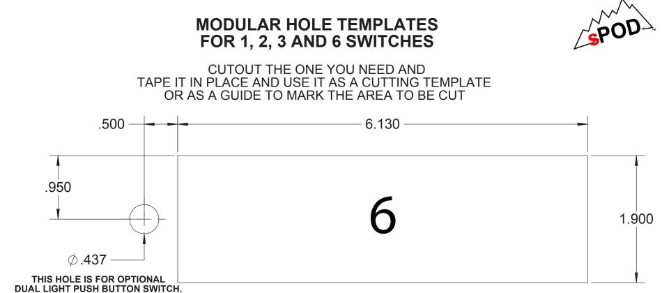
MAX. PANEL THICKNESS IS 3/32" (.093) THICK
